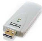
When RF Receivers are used near each other, each Receiver needs to be set on its own channel.
